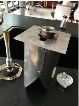
3. NEXT to the calorimeter (NOT inside), light the marshmallow on fire with the burner. When the marshmallow ignites, push the contraption under the calorimeter.
